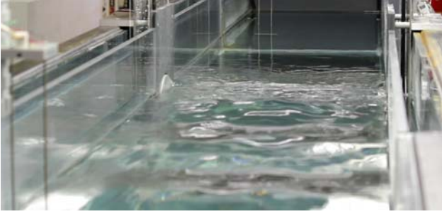
Figure 4. Picture of water surface for wave generation using a single bladed wave energy converter. Wave Period T = 0.55s , blade pitch \alpha = -7.5^\circ , submergence |y_c| - R = 15mm .
