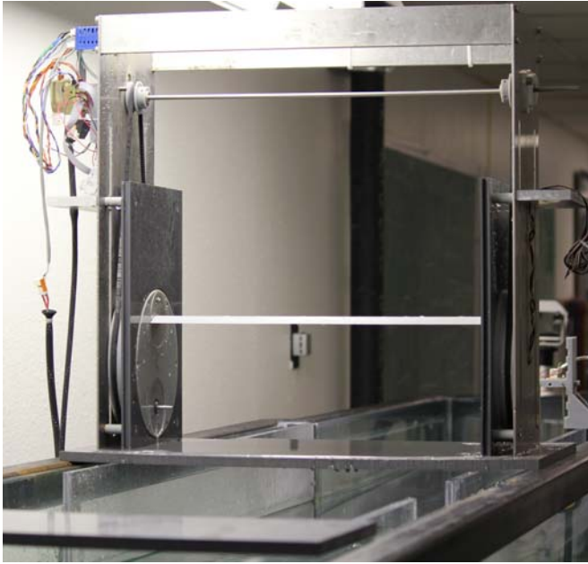
Figure 3. Picture of wave energy converter with a single blade installed.
