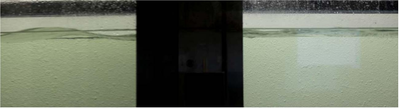
Fig. 5. Picture of wave cancellation from side. Incoming wave period  $T = 0.5s$ , flap wave maker amplitude  $\delta = 1.5$ , WEC has two blades, feedback phase  $\theta = 197^\circ$ , blade pitch gain  $G_p = 400^\circ/m$ , submergence  $|y_c| - R = 15mm$ .
