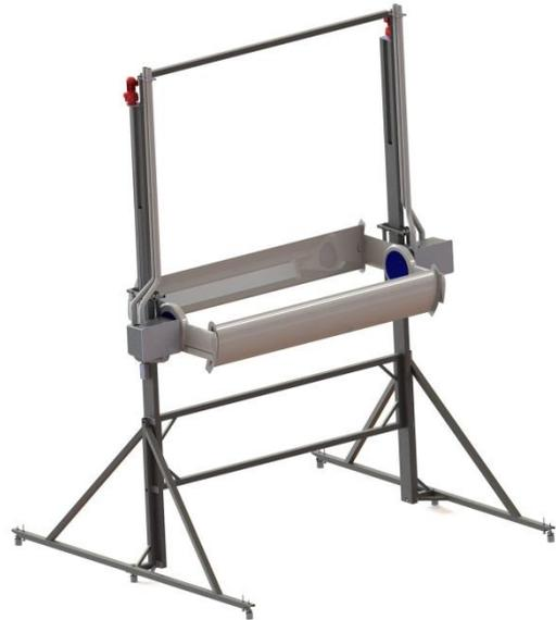
Figure 3: CAD model of CycWEC 1:10 scale model on floor mount
