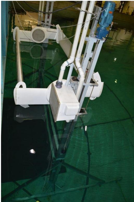
Figure 4: CycWEC 1:10 scale model installed in OTRC wave tunnel. The WEC is lifted above the water line during installation in this picture.
