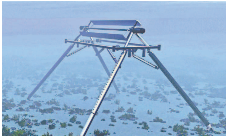
Pueblo's Atargis has developed the CycWEC which uses cycloidal wave energy conversion below the water surface to generate power.
